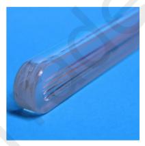
side (medium side) are imprinted longitudinal grooves (3 or 4), which walls are angled to each other at an angle of 90°. Squeezing process causes the formation of grooves. On the surface of the grooves creates extremely smooth and hard glass layer, very resistant to the environment. With the grooving increases the angle of refraction which makes the visibility of the liquid level is much better than when using smooth glass. **For reflective glass does not apply mica shields**.
